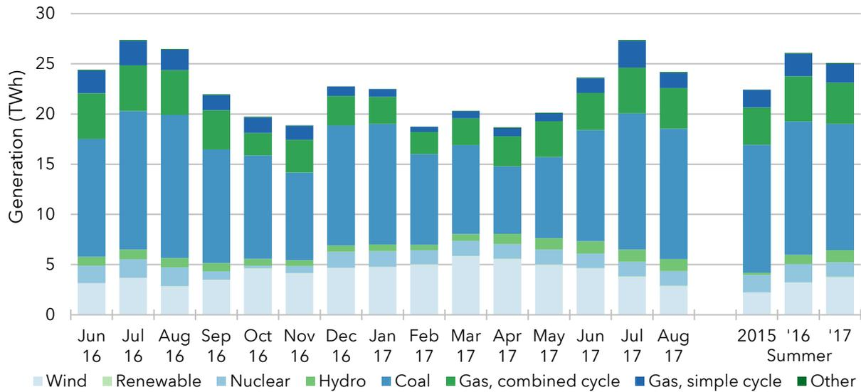
As shown in Figure 3–6 below real-time market generation by coal-powered resources continues a downward trend representing only 50 percent of total energy produced in the summer 2017 period, compared to 57 percent in 2015. This decline has been primarily offset by increases in wind generation, which is up from 10 percent in summer 2015 to 15 percent in 2017.
