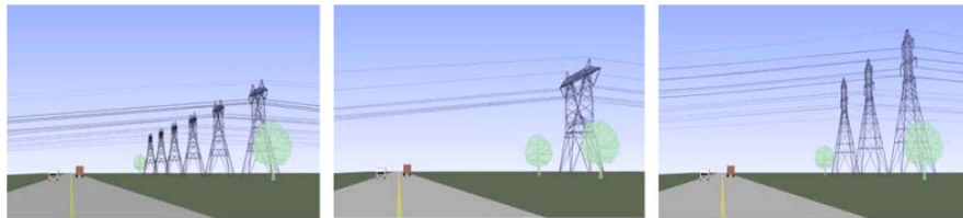
345 kV Six Single Circuit Towers (900 ft. Right-of-Way)
